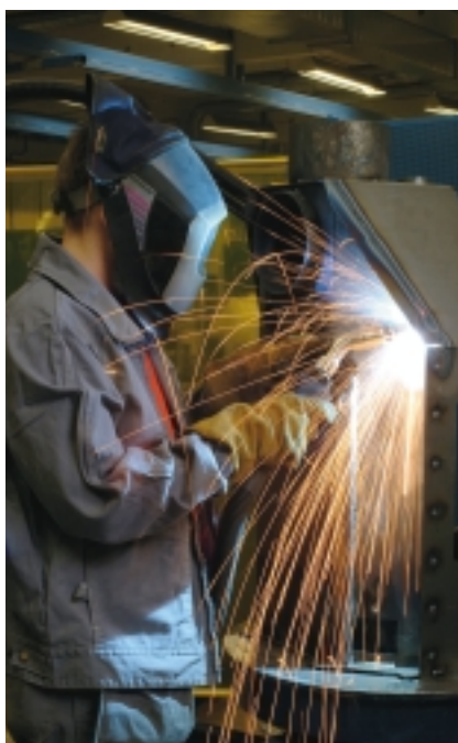
Most of the work on wood-burning stoves is carried out by welding robots, although some critical operations are performed manually.
