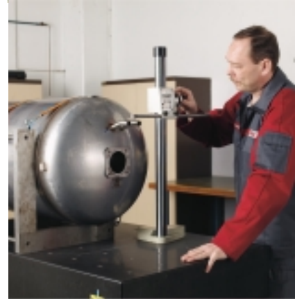
X-ray control of welds for water heaters and dimension controls are both part of the quality assurance procedures at NIBE Heating.
